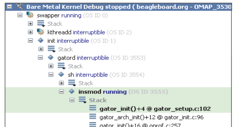
DS-5 supports Linux kernel and driver debugging, and shows resources and dynamically loaded modules.
