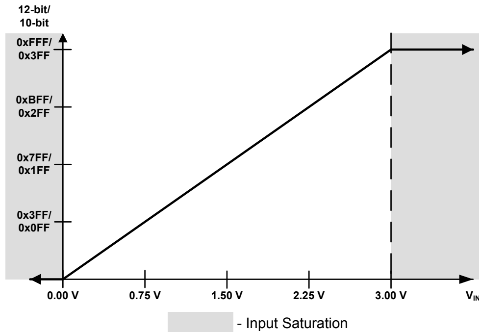
Figure 12-8. Internal Voltage Conversion Result
