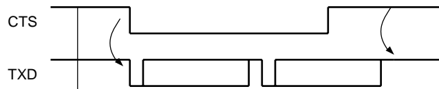
Figure 107. Transmitter Behavior when Operating with Hardware Handshaking
