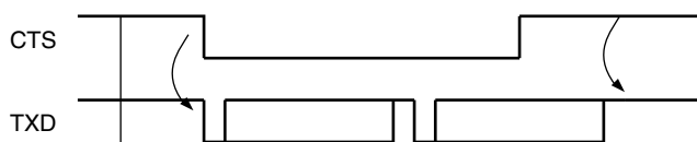
Figure 39-28. Transmitter Behavior when Operating with Hardware Handshaking
