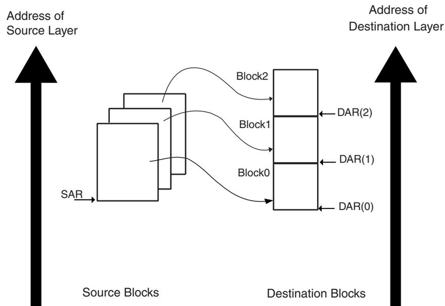
**Figure 24-13.** DMA Transfer for Source Address Auto-reloaded and Contiguous Destination Address
