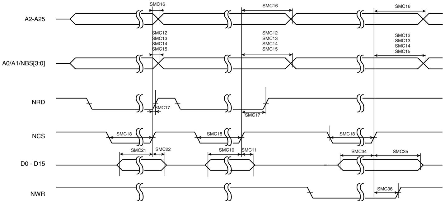
Figure 46-3. SMC Signals for NRD and NWR Controlled Accesses
