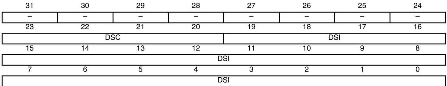
The address offset for each channel is:  $0x50 + [x * 0x58]$
