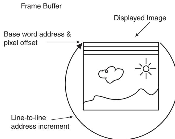
In order to locate the displayed window within a larger frame buffer, the software must:
