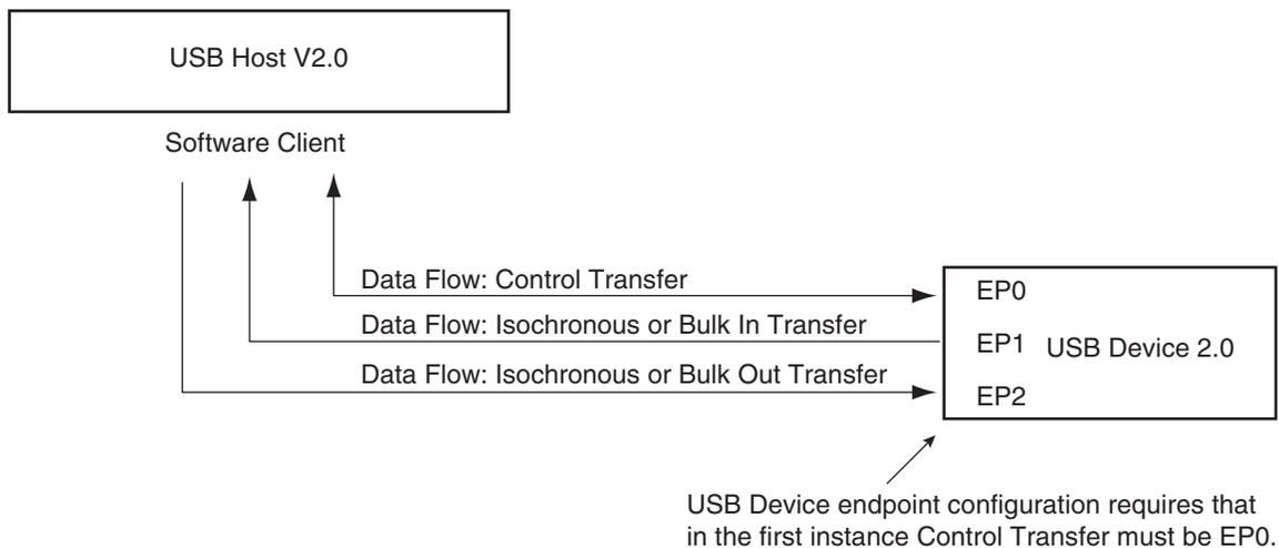
The Control Transfer endpoint EP0 is always used when a USB device is first configured (USB v. 2.0 specifications).
