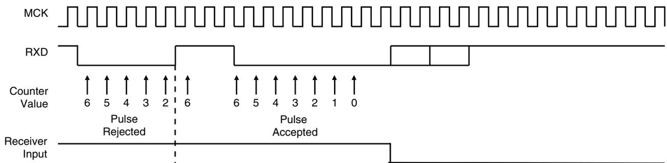
As the IrDA mode uses the same logic as the ISO7816, note that the FI\_DI\_RATIO field in US\_FIDI must be set to a value higher than 0 in order to assure IrDA communications operate correctly.
