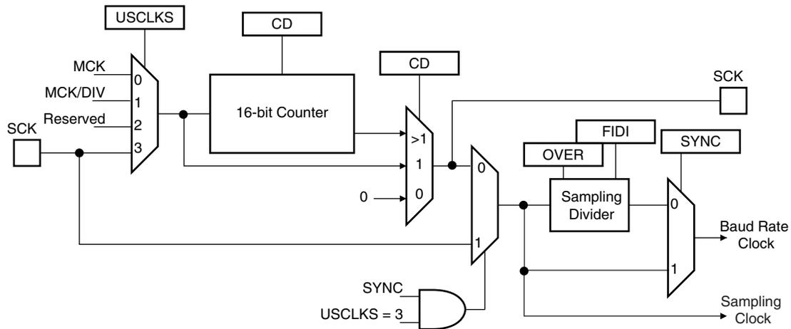
**33.6.1.1 Baud Rate in Asynchronous Mode**
