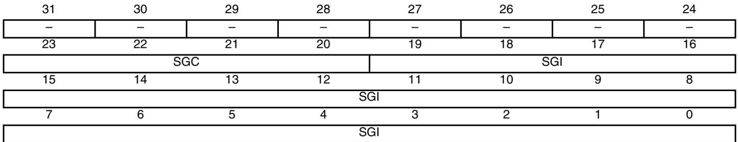
The address offset for each channel is:  $0x48 + [x * 0x58]$
