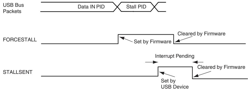
**Figure 42-14.** Stall Handshake (Data OUT Transfer)
