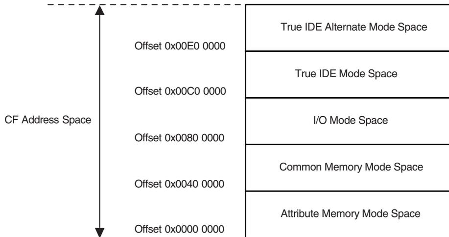
Note: The A22 pin is used to drive the REG signal of the CompactFlash Device (except in True IDE mode).
