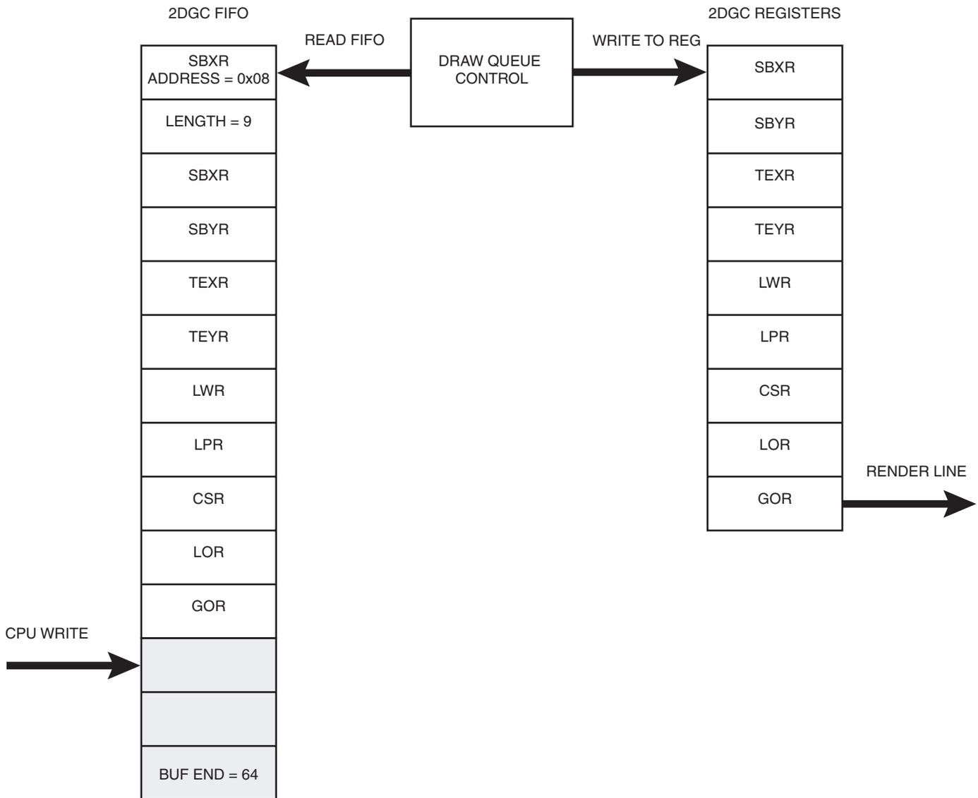
*Recommended Procedure for Using the Command Queue*
