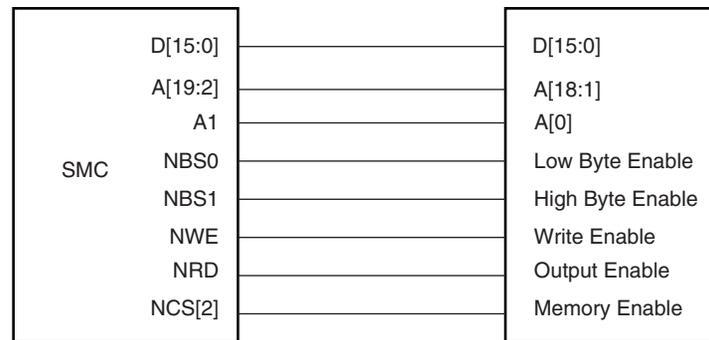
**Figure 21-5.** Memory Connection for a 32-bit Data Bus
