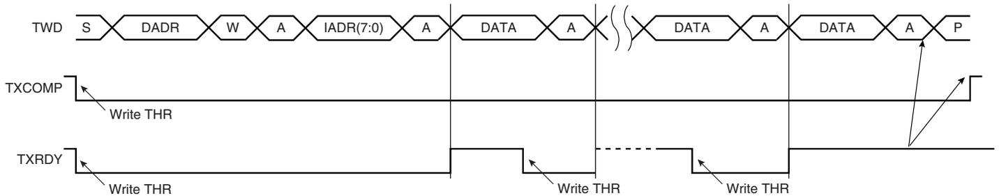
**Figure 32-7. Master Read with One, Two or Three Bytes Internal Address and One Data Byte**
