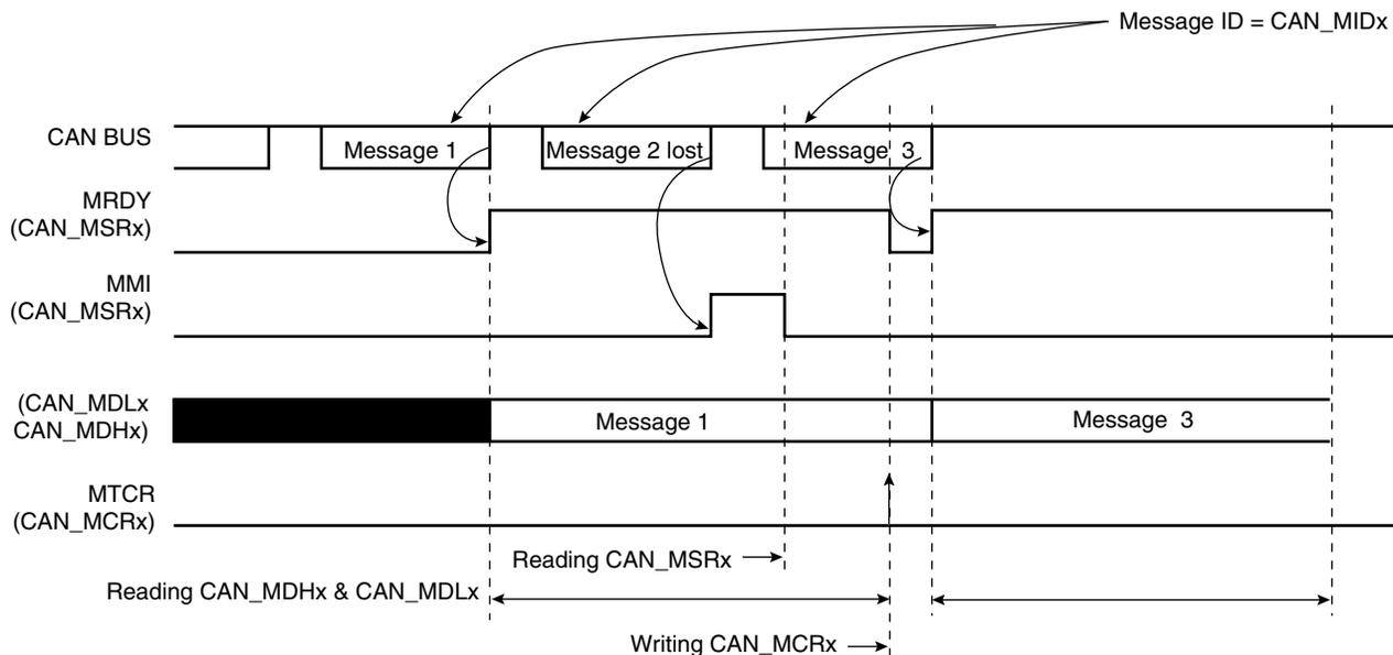
Note: In the case of ARM architecture, CAN\_MSRx, CAN\_MDLx, CAN\_MDHx can be read using an optimized Idm assembler instruction.
