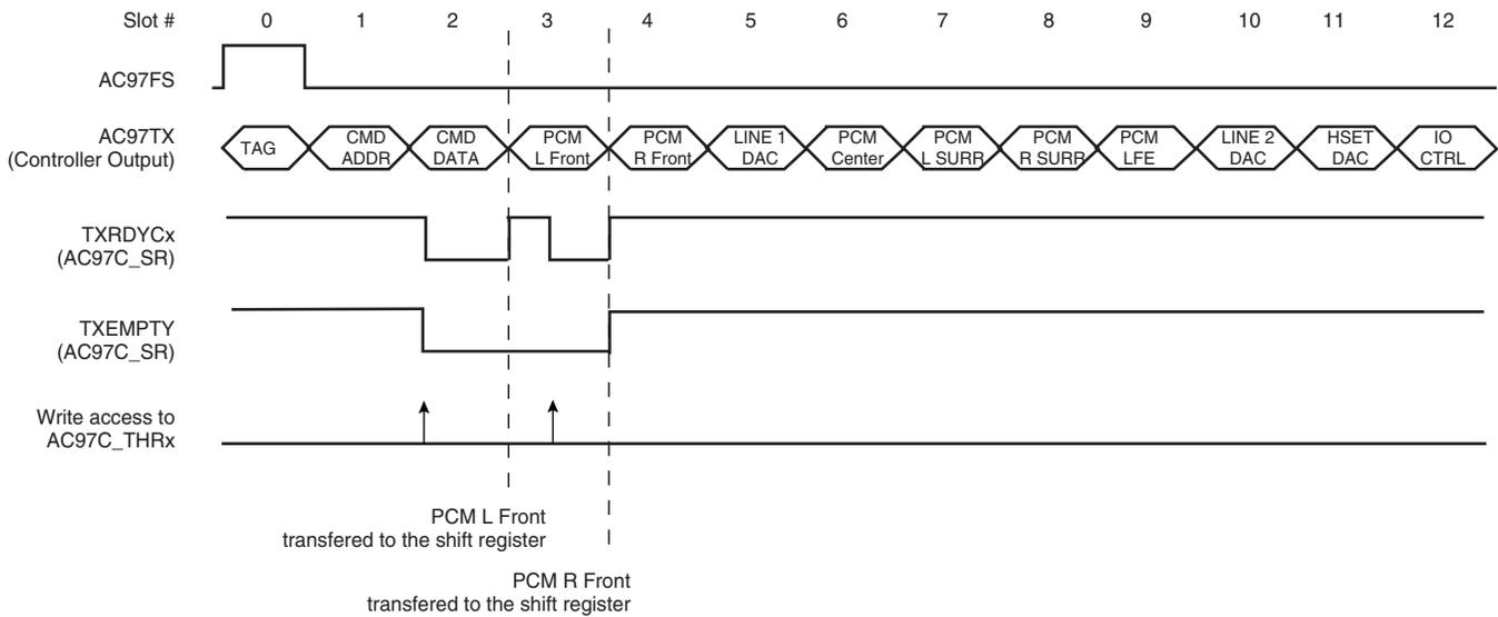
The TXEMPTY flag in the AC'97 Controller Channel x Status Register (AC97C\_CxSR) is set when all requested transmissions for a channel have been shifted on the AC-link. The application can either poll TXEMPTY flag in AC97C\_CxSR or wait for an interrupt notice associated with the same flag.
