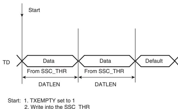
Note: 1. STTDLY is set to 0. In this example, SSC\_THR is loaded twice. FSDEN value has no effect on the transmission. SyncData cannot be output in continuous mode.
