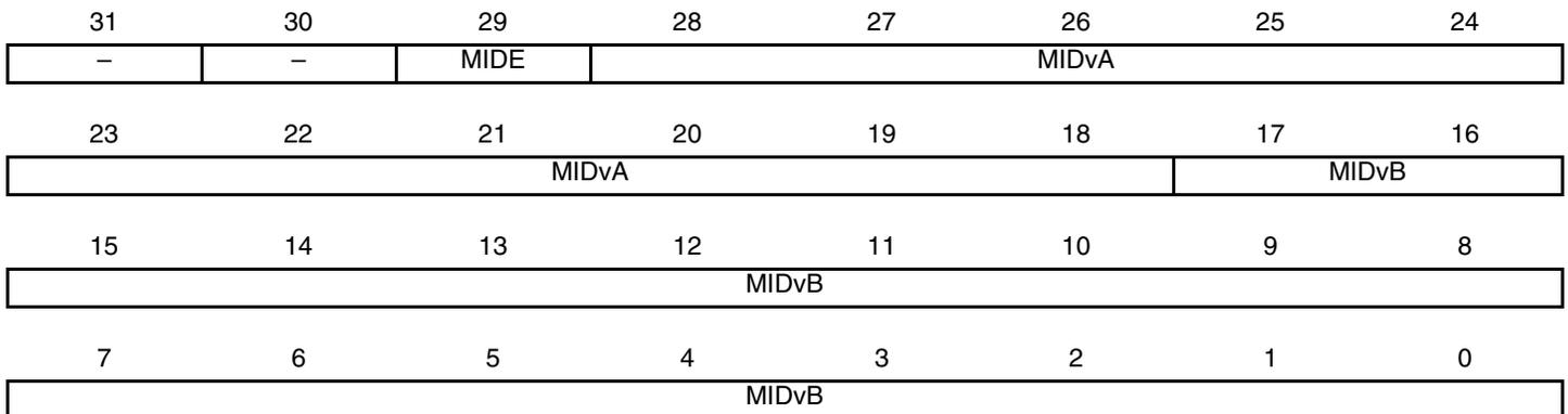
To prevent concurrent access with the internal CAN core, the application must disable the mailbox before writing to CAN\_MIDx registers.
