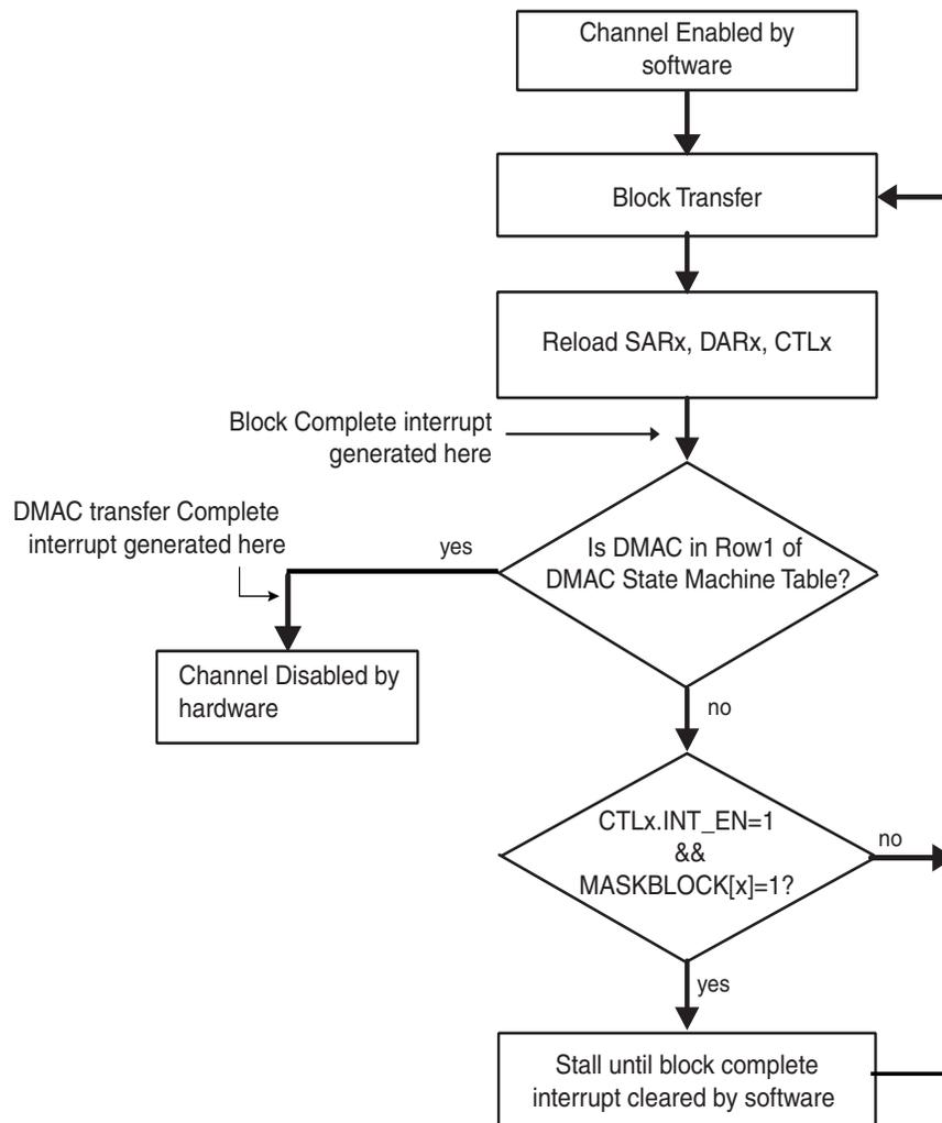
*Multi-block Transfer with Source Address Auto-reloaded and Linked List Destination Address (Row7)*
