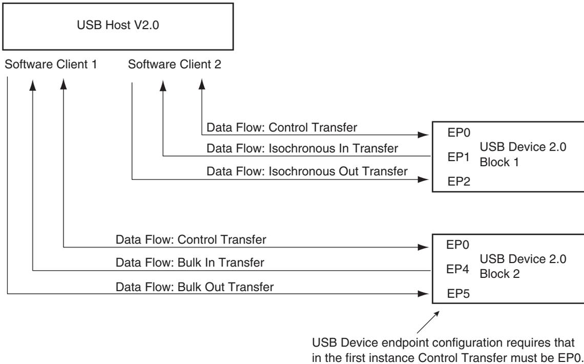
**Figure 42-4.** Example of USB V2.0 Full-speed Communication Control
