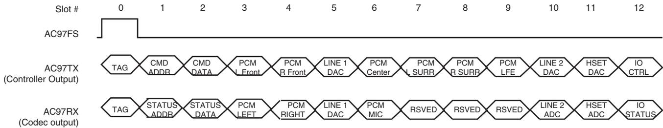
**Table 35-2.** AC-link Output Slots Transmitted from the AC'97C Controller
