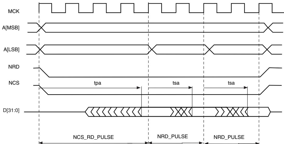
The NRD and NCS signals are held low during all read transfers, whatever the programmed values of the setup and hold timings in the User Interface may be. Moreover, the NRD and NCS timings are identical. The pulse length of the first access to the page is defined with the
