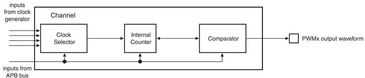
Each of the **X** channels is composed of three blocks:
