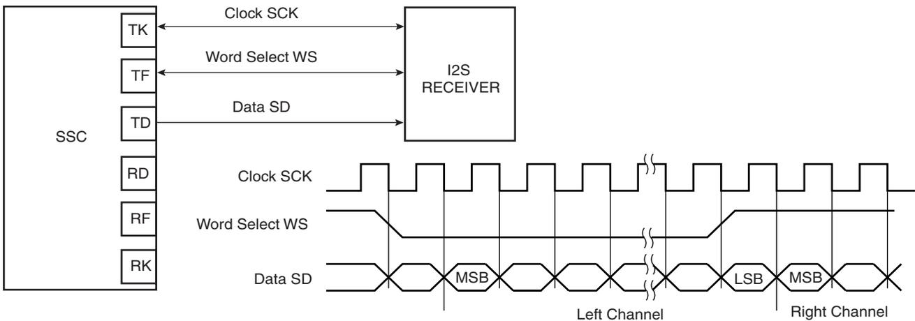
**Figure 34-18. Codec Application Block Diagram**
