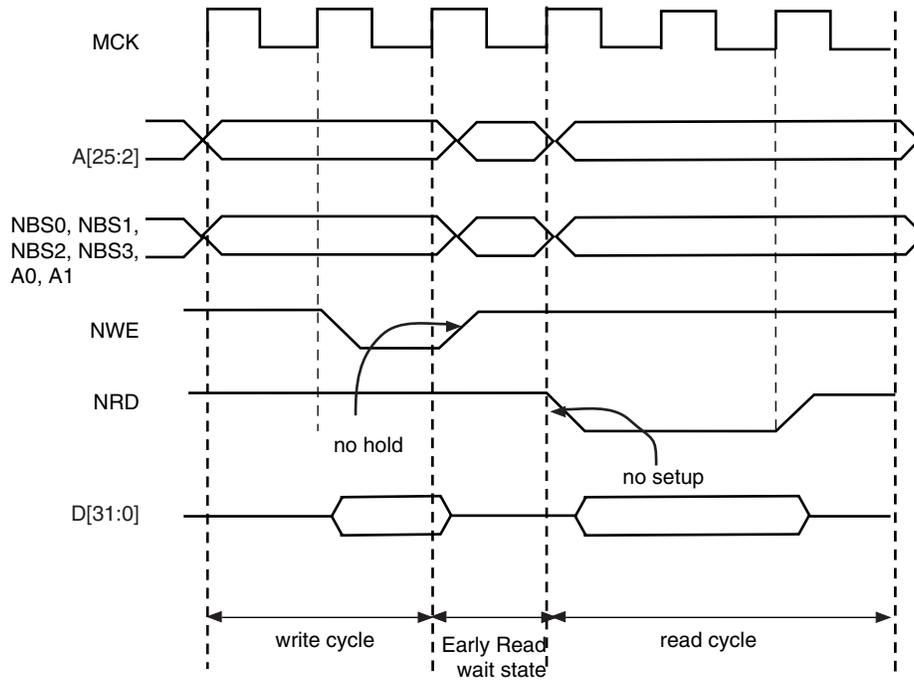
**Figure 21-18.** Early Read Wait State: NCS Controlled Write with No Hold Followed by a Read with No NCS Setup
