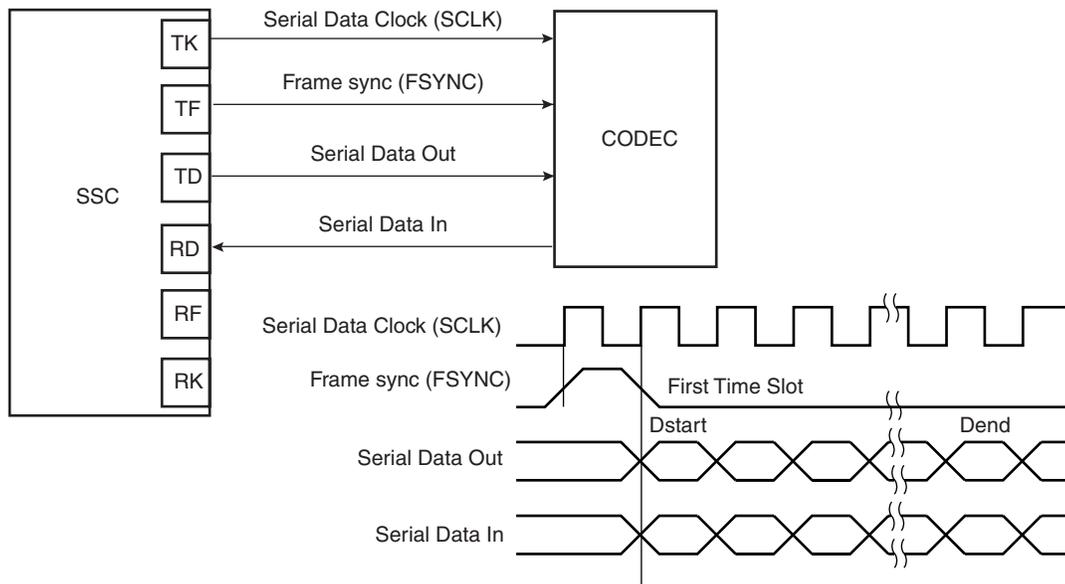
**Figure 34-19. Time Slot Application Block Diagram**
