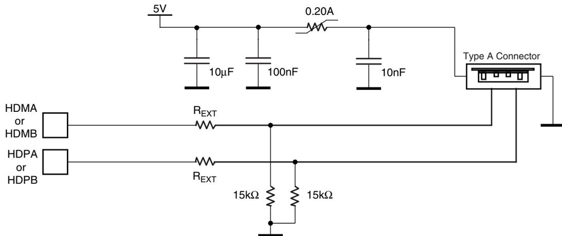
As device connection is automatically detected by the USB host port logic, a pull-down must be connected on DP and DM on the board. Otherwise the USB host permanently detects a device connection on this port.
