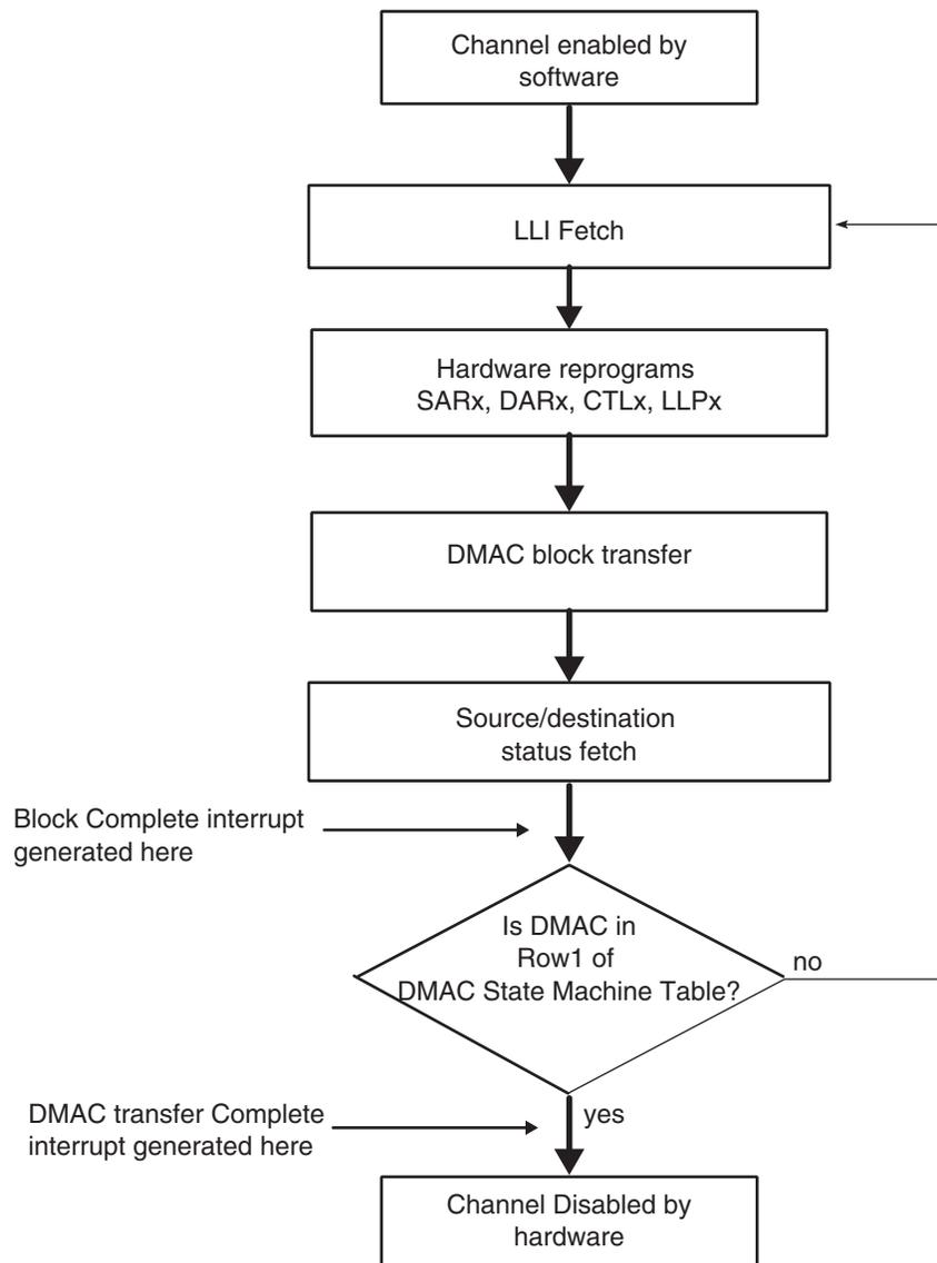
*Multi-block Transfer with Source Address Auto-reloaded and Destination Address Auto-reloaded (Row 4)*
