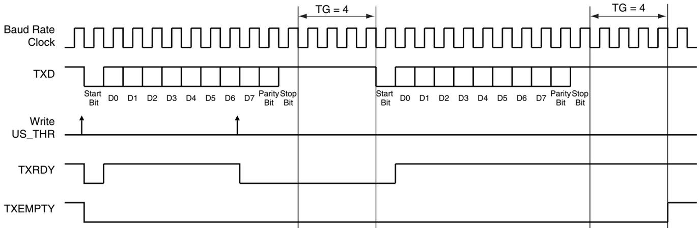
Table 33-7 indicates the maximum length of a timeguard period that the transmitter can handle in relation to the function of the Baud Rate.
