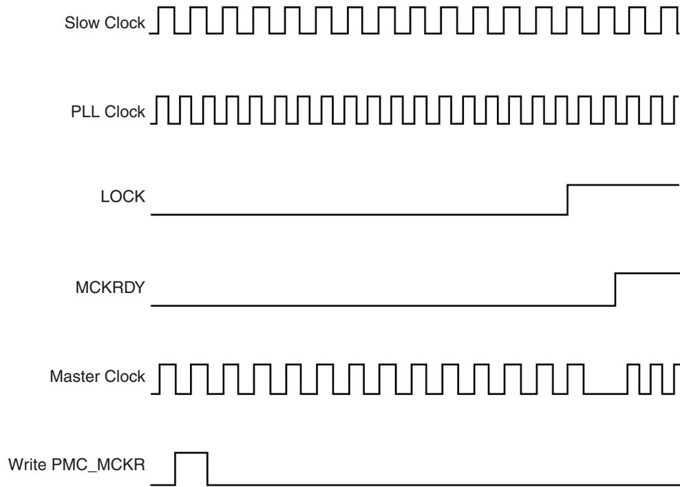
**Figure 27-4.** Switch Master Clock from Main Clock to Slow Clock
