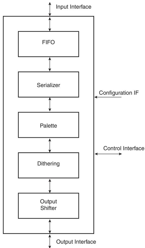
This module transforms the data read from the memory into a format according to the LCD module used. It has four different interfaces: the input interface, the output interface, the configuration interface and the control interface.
