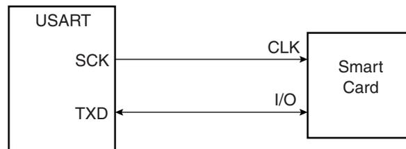
When operating in ISO7816, either in T = 0 or T = 1 modes, the character format is fixed. The configuration is 8 data bits, even parity and 1 or 2 stop bits, regardless of the values programmed in the CHRL, MODE9, PAR and CHMODE fields. MSBF can be used to transmit LSB or MSB first. Parity Bit (PAR) can be used to transmit in normal or inverse mode. Refer to [“USART Mode Register” on page 518](#) and [“PAR: Parity Type” on page 519](#).
