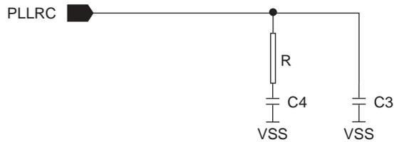
The optimum response with a simple RC filter is obtained when:
